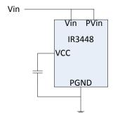
Figure 16: Internally Biased Single Supply Configuration
