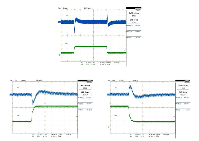
Figure 37: Vout Transient Response, 1.6A to 6.4A step at 2.5A/uSec CH2:Vout, CH4:lout
