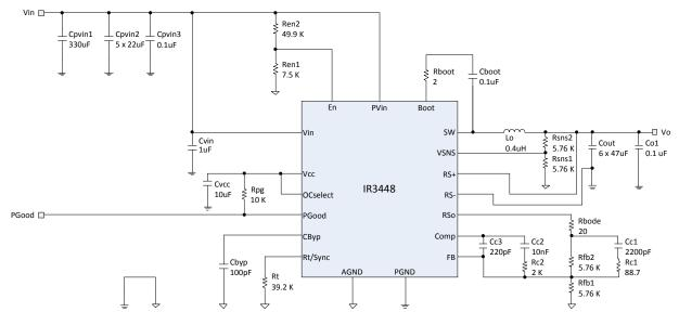
Figure 28: Application circuit for a 12V to 1.2V, 16A Point of Load Converter Using the Internal LDO
