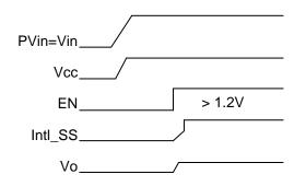
Figure 5: Recommended startup for Normal operation
