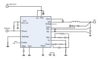
Figure 1: IR3448 Basic Application Circuit
