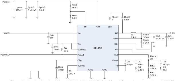
Figure 29: Application circuit for a 12V to 1.2V, 13A Point of Load Converter using external 5V VCC
