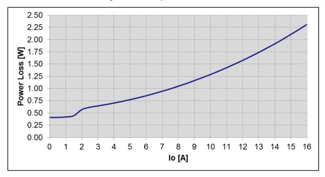
Figure 41: Power Loss versus load current
