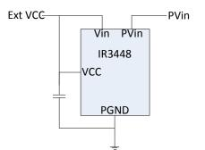
Figure 17: Externally Biased Configuration
