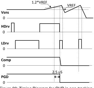
Figure 20: Timing Diagram for OVP in non-tracking mode
