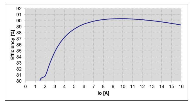
Figure 40: Efficiency versus load current
