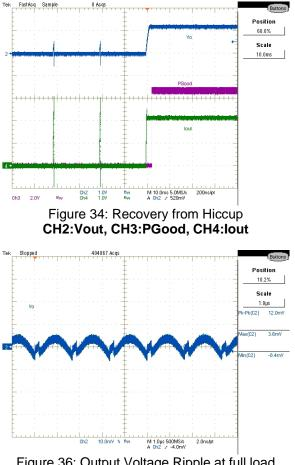
Figure 36: Output Voltage Ripple at full load CH1:Vout
