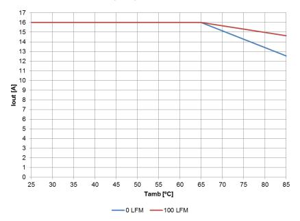
Note: International Rectifier Corporation specifies current rating of SupIRBuck devices conservatively. The continuous current load capability might be higher than the rating of the device if input voltage is 12V typical and switching frequency is below 600kHz. However, the maximum current is limited by the internal current limit and designers need to consider enough guard bands between load current and minimum current limit to guarantee that the device does not trip at steady state condition.
