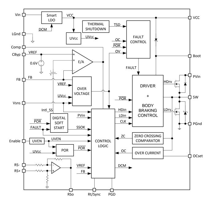
Figure 3: IR3448 Simplified Block Diagram
