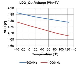
Figure 18: LDO\_Out Voltage in dropout mode
