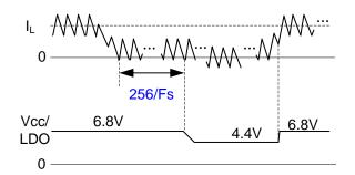
Figure 14: Time Diagram for Smart LDO
