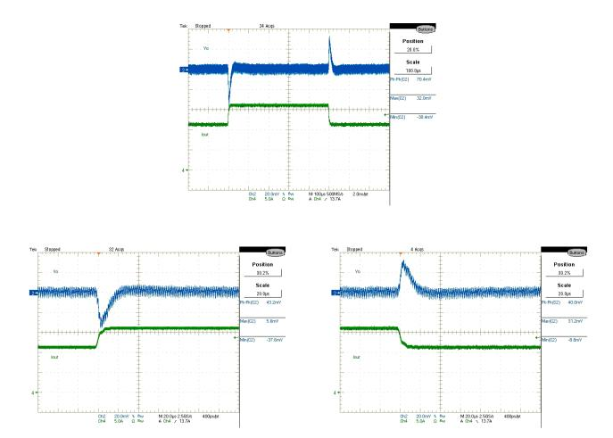
Figure 38: Vout Transient Response, 11.2A to 16A step at 2.5A/uSec CH2:Vout, CH4:lout
