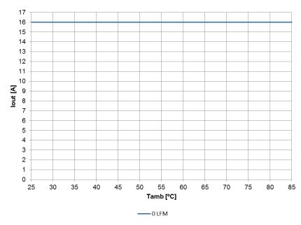
Vin=PVin=12V, Vout =1.2V, VCC=internal LDO (6.8V), Fs = 600kHz
